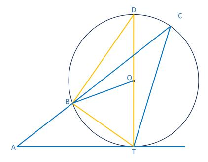
Third we note that  $\angle ATD$  is a right angle because the line TD is perpendicular to AT.
