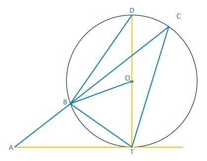
Fourth we can now calculate  $\angle ATB$ :  $\angle ATB + \angle BTD$  is 90°; and  $\angle BTD + \angle TDB$  is 90°, so  $\angle ATB = \angle TDB$ , which from the first stage we know equals  $\angle TCB$ . Hence  $\angle ATB = \angle TCB$ .
